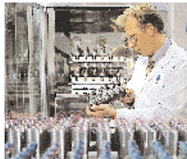
Computerized testing and calibration of pressure transducers.
